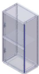
Armadio con apertura ante invertita Enclosure with 2 compartments with reversed door opening
